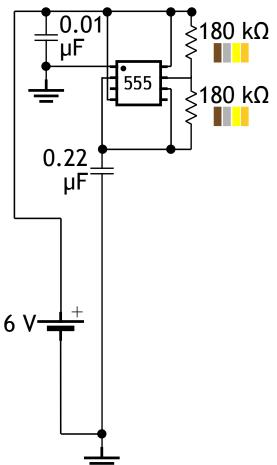
Just the clock first: This is same 555 circuit as last week, just with different resistors (and therefore a different frequency).
