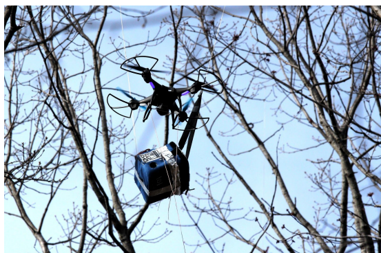
Figure-14 (left): The drone hauling a rope across the payload stranded 50 feet up on a tree
