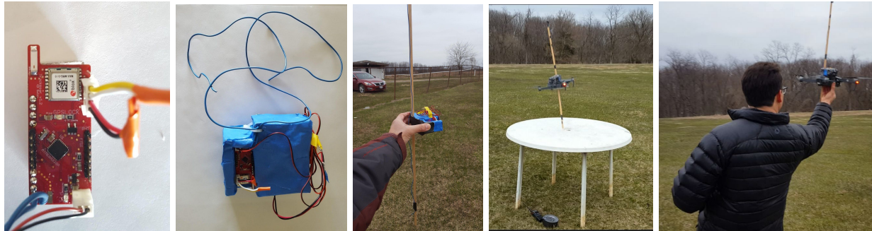
Figure-6 (left to right): a. Tracksoar outside its protective casing. b. Tracksoar nestled inside its styrofoam casing with attachments for the battery and the dipole antenna c. Tracksoar in a custom built styrofoam casing with the dipole antenna held vertical using Balsa wood. This configuration was used to execute the APRS I-Gate repeater test using a Drone. d. The drone with Tracksoar taking off to reach an altitude of 400 ft. e. Dom Perez from CASA (Capital Area Soaring Association) catching the expensive drone in the air since it couldn't land without damaging itself due to the antenna setup
