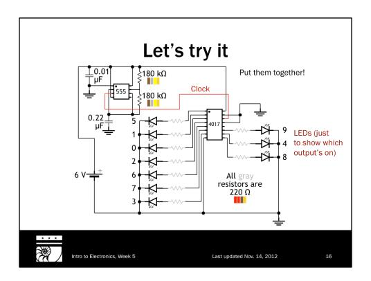
The only thing you need to put these two together is one more wire going from the timer's output pin (pin 3) to the counter's clock pin (pin 14). It's the connection highlighted in red.
