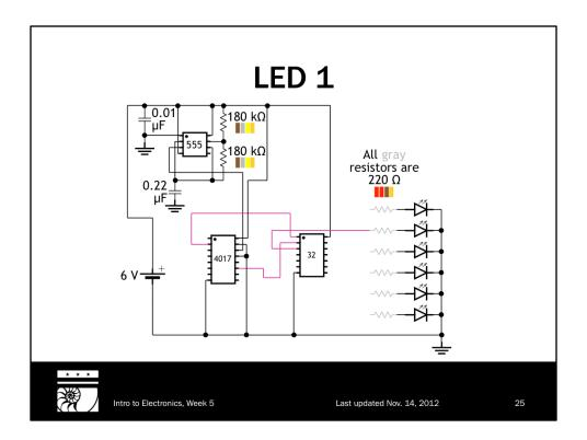
I'll highlight one OR gate's connections at a time. For each of these, there'll be two wires going from the counter to the OR gate and one wire going from the OR gate to an LED's resistor.
