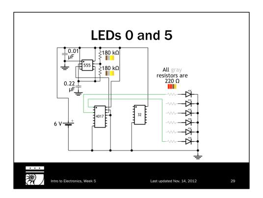
There are two more LEDs to worry about — the ones at either end of the string. These only turn on at one point each in the sequence, so we can just connect them directly to the counter rather than doing anything with OR gates. (That's good, because we're out of OR gates.)
