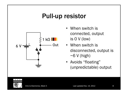
When the switch is connected, the output is at 0 V because all of the batteries' 6 V ends up going across the resistor. (This means it does draw current from the battery — 6 mA, specifically. (Remember how to do that?) Much like the filter capacitor last week that just went between positive and negative, this is the sort of thing where you just pick a reasonable size because (within reason) it doesn't really matter what specific value you use.)
