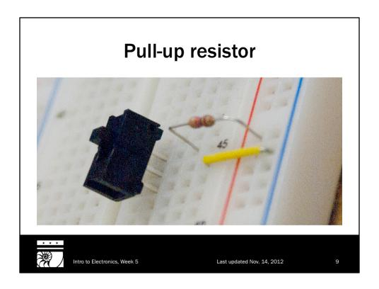
(Yes, I know that because we have an SPDT switch, we could connect the middle terminal to the output and the other two terminals to positive and negative and theoretically be able to get rid of the resistor. If you just had a plain (SPST) switch that has only two terminals, though, and can just connect or disconnect them, you'd definitely need something like this.)
