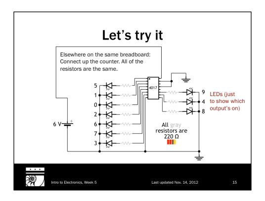
Useful thing to notice: The counter has four connections to power. The top right pin (pin 16) goes to the positive supply, the bottom left pin (pin 8) goes to the negative (ground), and two of the other pins on the chip (pins 13 and 15, which control other details about how the counter runs) also go to ground. (Remember, pins on chips are numbered starting with pin 1 at the dot and going up as you go counterclockwise.)
