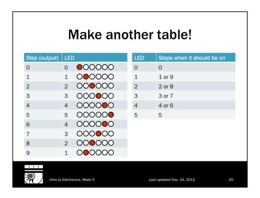
Each LED has one or two times in the sequence when it needs to be turned on.
