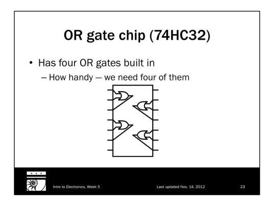
The two remaining pins are for positive (top right, pin 14) and ground (bottom left, pin 7). This is a really common thing for logic chips. (Remember that the counter had the same setup.)
