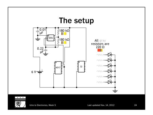
Let's start by setting all of the chips and LEDs up where we want them and then focus on the connections between them. (I've broken up all of those connections into the next several slides so it's not so overwhelming.)
