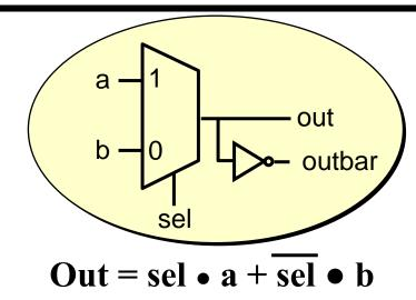
2-to-1 multiplexer with inverted output
